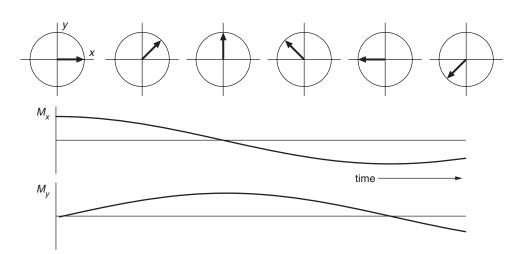
Fig. 4.2 Evolution of the magnetization over time; the offset is assumed to be positive and the magnetization starts out along the x axis.
