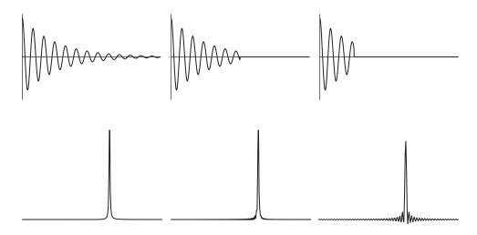
Fig. 4.15 Illustration of how truncation leads to artefacts (called *sinc wiggles*) in the spectrum. The FID on the left has been recorded for sufficient time that it has decayed almost the zero; the corresponding spectrum shows the expected lineshape. However, if data recording is stopped before the signal has fully decayed the corresponding spectra show oscillations around the base of the peak.
