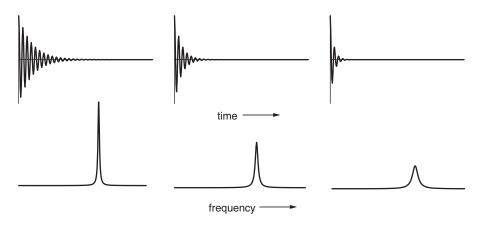
Fig. 4.6 Illustration of the fact that the more rapidly the FID decays the broader the line in the corresponding spectrum. A series of FIDs are shown at the top of the figure and below are the corresponding spectra, all plotted on the same vertical scale. The integral of the peaks remains constant, so as they get broader the peak height decreases.
