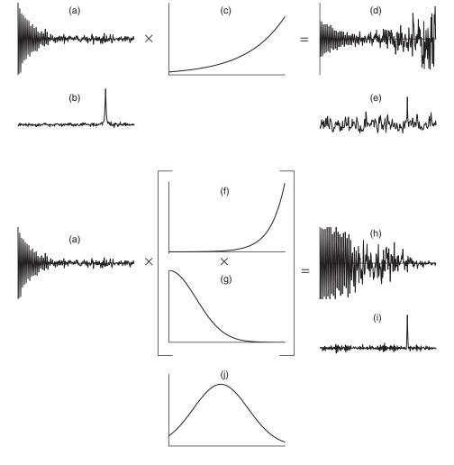
Fig. 4.11 Illustration of the use of weighting functions to enhance the resolution in the spectrum. Note that the scales of the plots have been altered to make the relevant features clear. See text for details.
