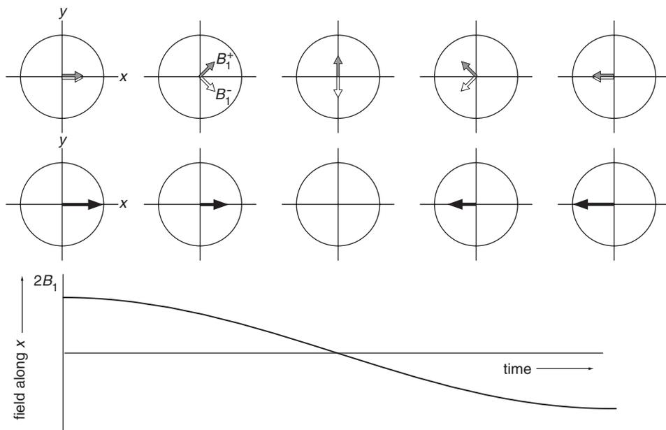
Fig. 3.8 Illustration of how two counter-rotating fields (shown in the upper part of the diagram and marked  $B_1^+$  and  $B_1^-$ ) add together to give a field which is oscillating along the x axis (shown in the lower part). The graph at the bottom shows how the field along x varies with time.
