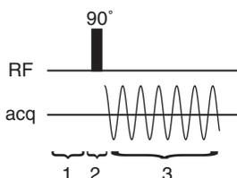
**Fig. 3.15** Timing diagram or pulse sequence for the simple pulse–acquire experiment. The line marked “RF” shows the location of the pulses, and the line marked “acq” shows when the signal is recorded or *acquired*.
