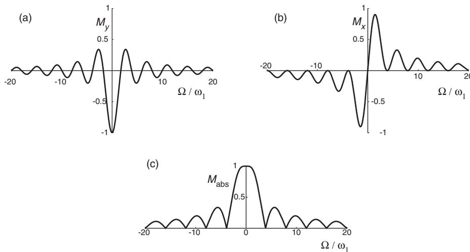
**Fig. 3.26** Plots of the magnetization produced by a pulse as a function of the offset. The pulse length has been adjusted so that on resonance the flip angle is  $90^\circ$ . The horizontal axes of the plots is the offset expressed as a ratio of the RF field strength,  $\omega_1$ ; the equilibrium magnetization has been assumed to be of size 1.
