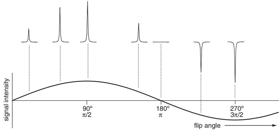
**Fig. 3.18** Illustration of how pulse calibration is achieved. The signal intensity varies as  $(\sin \beta)$  as shown by the curve at the bottom of the picture. Along the top are the spectra which would be expected for various different flip angles (indicated by the dashed lines). The signal is a maximum for a flip angle of  $90^\circ$  and goes through a null at  $180^\circ$ ; after that, the signal goes negative.
