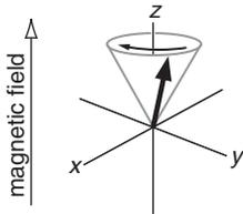
**Fig. 3.2** If the magnetization vector is tilted away from the  $z$  axis it executes a precessional motion in which the vector sweeps out a cone of constant angle to the magnetic field direction. The direction of precession shown is for a nucleus with a positive gyromagnetic ratio and hence a negative Larmor frequency.
