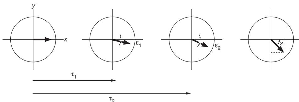
Fig. 3.5 Illustration of the precession of the magnetization vector in the  $xy$ -plane. The angle through which the vector has precessed is given by  $\omega_0 t$ . On the right-hand diagram we see the geometry for working out the  $x$  and  $y$  components of the vector.
