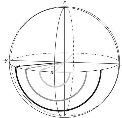
**Fig. 3.21** Illustration of the effect of a  $180^\circ$  pulse on three vectors which start out at different angles from the  $-y$  axis (coloured in black, grey and light grey). All three are rotated by  $180^\circ$  about the  $x$  axis on the trajectories indicated by the thick lines which dip into the southern hemisphere. As a result, the vectors end up in mirror image positions with respect to the  $xz$ -plane.
