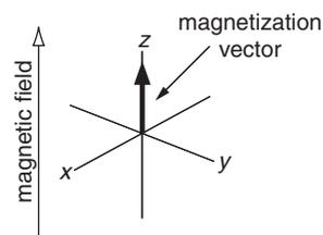
**Fig. 3.1** At equilibrium, a sample has a net magnetization along the magnetic field direction (the  $z$  axis) which can be represented by a magnetization vector. The axis set in this diagram is a right-handed one, which is what we will use throughout these lectures.
