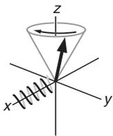
**Fig. 3.3** The precessing magnetization will cut a coil wound round the  $x$  axis, thereby inducing a current in the coil. This current can be amplified and detected; it is this that forms the free induction signal. For clarity, the coil has only been shown on one side of the  $x$  axis.
