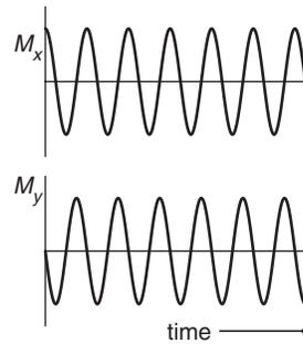
**Fig. 3.6** Plots of the  $x$ - and  $y$ -components of the magnetization predicted using the approach of Fig. 3.5. Fourier transformation of these signals will give rise to the usual spectrum.
