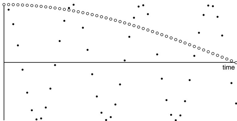
The open circles lie on a cosine wave,  $\cos(\Omega \times n\Delta)$ , where  $\Delta$  is the sampling interval and  $n$  runs 0, 1, 2 ... The closed circles lie on a cosine wave in which an additional phase is incremented on each point *i.e.* the function is  $\cos(\Omega \times n\Delta + n\phi)$ ; here  $\phi = \pi/8$ . The way in which this phase increment increases the frequency of the cosine wave is apparent.
