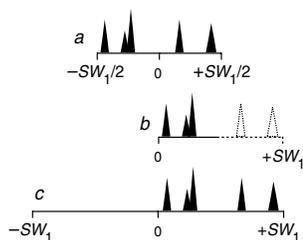
Illustration of the TPPI method. The normal spectrum is shown in a, with peaks in the range  $-SW/2$  to  $+SW/2$ . Adding a frequency of  $SW/2$  to all the peaks gives them all positive offsets, but some, shown dotted) will then fall outside the spectral window – spectrum b. If the spectral width is doubled all peaks are represented correctly – spectrum c.
