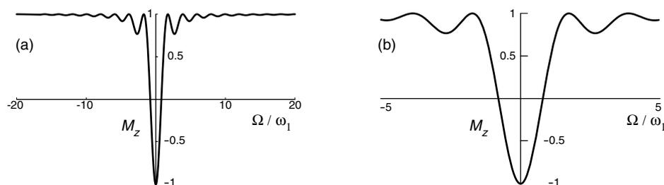
**Fig. 3.28** Plots of the  $z$ -magnetization produced by a pulse as a function of the offset; the flip angle on-resonance has been set to  $180^\circ$ . Plot (b) covers a narrower range of offsets than plot (a). These plots should be compared with those in Fig. 3.26.
