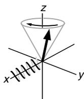
**Fig. 3.3** The precessing magnetization will cut a coil wound round the  $x$  axis, thereby inducing a current in the coil. This current can be amplified and detected; it is this that forms the free induction signal. For clarity, the coil has only been shown on one side of the  $x$  axis.
