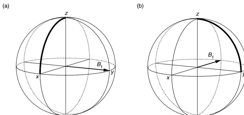
**Fig. 3.22** Grapefruit plots showing the effect on equilibrium magnetization of (a) a  $90^\circ$  pulse about the  $y$  axis and (b) a  $90^\circ$  pulse about the  $-x$  axis. Note the position of the  $B_1$  field in each case.
