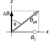
**Fig. 3.10** In the rotating frame the effective field  $B_{\text{eff}}$  is the vector sum of the reduced field  $\Delta B$  and the  $B_1$  field. The tilt angle,  $\theta$ , is defined as the angle between  $\Delta B$  and  $B_{\text{eff}}$ .
