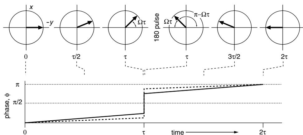
**Fig. 3.19** Vector diagrams showing how a spin echo refocuses the evolution of the offset; see text for details. Also shown is a phase evolution diagram for two different offsets (the solid and the dashed line).
