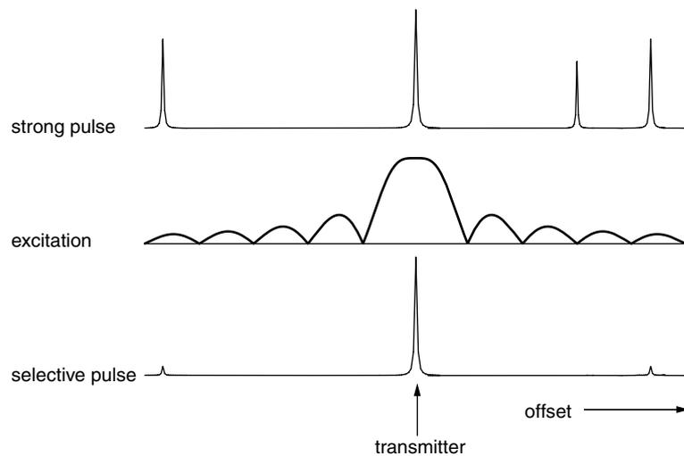
**Fig. 3.27** Visualization of the use of selective excitation to excite just one line in the spectrum. At the top is shown the spectrum that would be excited using a hard pulse. If the transmitter is placed on resonance with one line and the strength of the RF field reduced then the pattern of excitation we expect is as shown in the middle. As a result, the peaks at non-zero offsets are attenuated and the spectrum which is excited will be as shown at the bottom.
