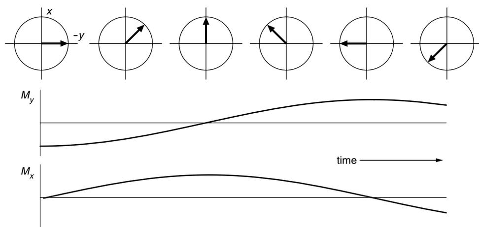
**Fig. 3.16** Evolution during the acquisition time (period 3) of the pulse–acquire experiment. The magnetization starts out along  $-y$  and evolves at the offset frequency,  $\Omega$  (here assumed to be positive). The resulting  $x$ - and  $y$ -magnetizations are shown below.
