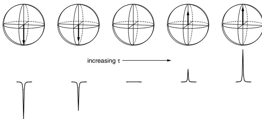
**Fig. 3.24** Visualization of the outcome of an inversion recovery experiment. The size and sign of the  $z$ -magnetization is reflected in the spectra (shown underneath). By analysing the peak heights as a function of the delay  $\tau$  it is possible to find the rate of recovery of the  $z$ -magnetization.
