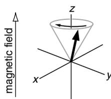
**Fig. 3.2** If the magnetization vector is tilted away from the  $z$  axis it executes a precessional motion in which the vector sweeps out a cone of constant angle to the magnetic field direction. The direction of precession shown is for a nucleus with a positive gyromagnetic ratio and hence a negative Larmor frequency.
