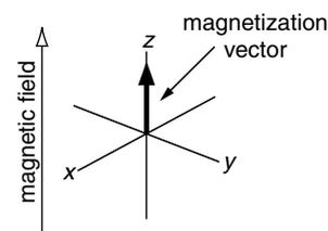
**Fig. 3.1** At equilibrium, a sample has a net magnetization along the magnetic field direction (the  $z$  axis) which can be represented by a magnetization vector. The axis set in this diagram is a right-handed one, which is what we will use throughout these lectures.
