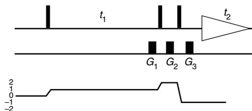
We use three gradients;  $G_1$  in  $t_1$  so as to select  $p = +1$  during  $t_1$ ;  $G_2$  to select double quantum during the filter delay and  $G_3$  to refocus prior to acquisition.
