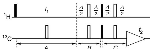
This sequence is closely related to HSQC, but differs in that the signal is observed on carbon-13, rather than being transferred back to proton for observation. Like HSQC and HMQC the resulting spectrum shows cross peaks whose co-ordinates are the shifts of directly attached carbon-13 proton pairs.
