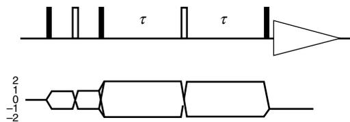
The  $180^\circ$  pulse placed in the middle of the double-quantum period is used to refocus evolution due to offsets and inhomogeneous line broadening.
